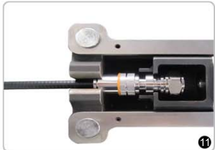
11 Make sure the connector and cable both lay flat in the compression frame.
